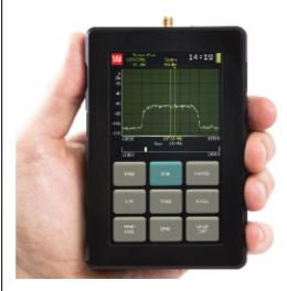
Spectrum Compact is the world's first powerful handheld licensed microwave spectrum analyzer. It is ultra light and easy to use measurement solution for 6 to 24 GHz licensed microwave frequency bands and designed especially for comfortable outdoor use by network engineers in a variety of challenging environments.
